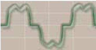
6-Pulse drives typically have distortion with steep current rises.
